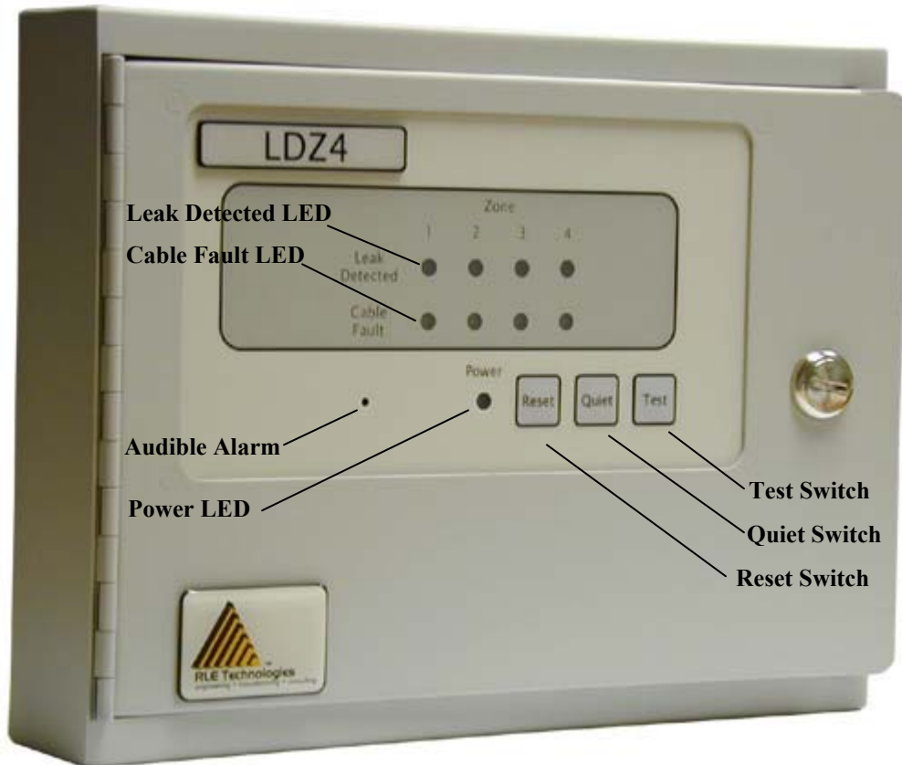
Figure 1-1: LDZ4 Front Panel Indicators
