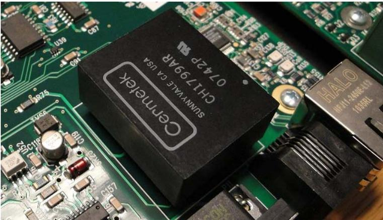
12. Look on both sides of the modem to ensure it is down evenly and the pins are inside the headers.
